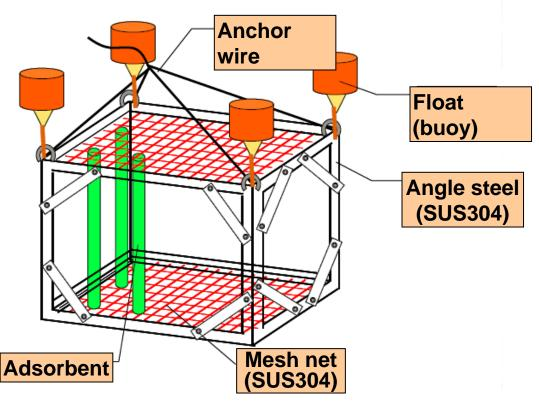
Fiber Adsorbent Purification Equipment
